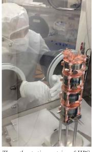
The author testing a string of HPGe detectors. The electroformed copper making up the detector mountings was grown and machined underground at the Davis Campus of SURF.
