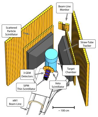
Figure 3: Rendering of the planned MUSE detector setup. The cartoon shows the setup as it is implemented in the MUSE simulation code, which our group has been developing. Our group is building the scintillation detectors (yellow) for the experiment at USC.
