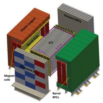
Figure 3: Schematic of the reference Near Detector of the DUNE experiment. The central Straw Tube Tracker (STT) is surrounded by a 4pi electromagnetic calorimeter (ECAL) placed inside a large aperture dipole magnet. Muon identification is provided by RPC located inside the iron yoke of the magnet and in the forward and backward regions.
