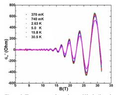
Figure 1: Temperature dependence of Shubnikov-de Haas oscillations in a sheet of graphene excised with an array of anti-dots. The isotherms are periodic in inverse magnetic fields and contain information about the Fermi-surface as well as quasi particle excitations.
