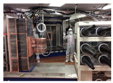
The Module 2 cryostat and 15,000-pound lead monolith (foreground) on its way from the assembly glovebox to its home in the main shield (background).
