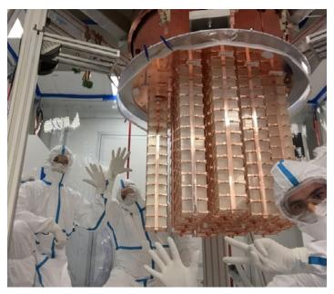
The recently completed CUORE bolometer array shown earlier with two towers left to install.
