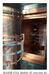
shield where Module #1 is visible in the
